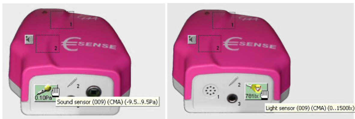
Figure 3. When a mouse cursor is located above the sensor icon Coach displays the sensor information: the sensor type and its measurement range.
